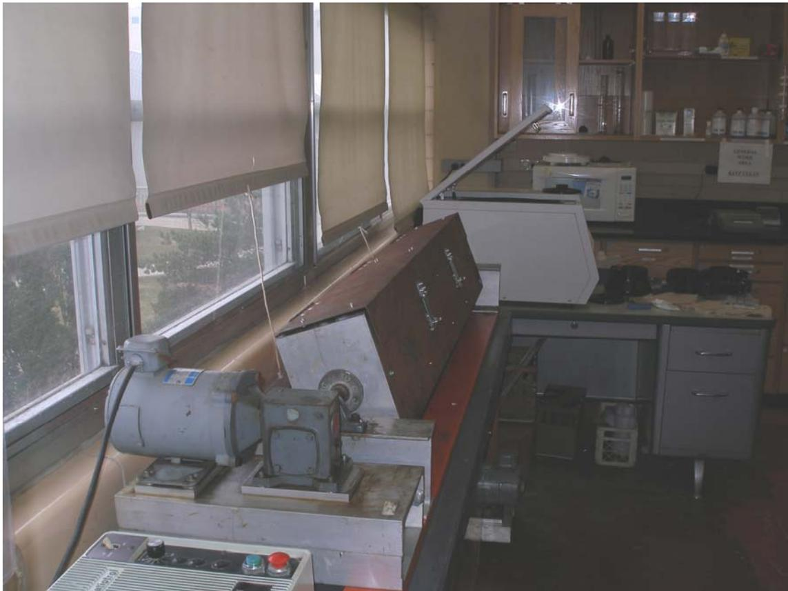
Fig. A-11. Water leach test rotator.
