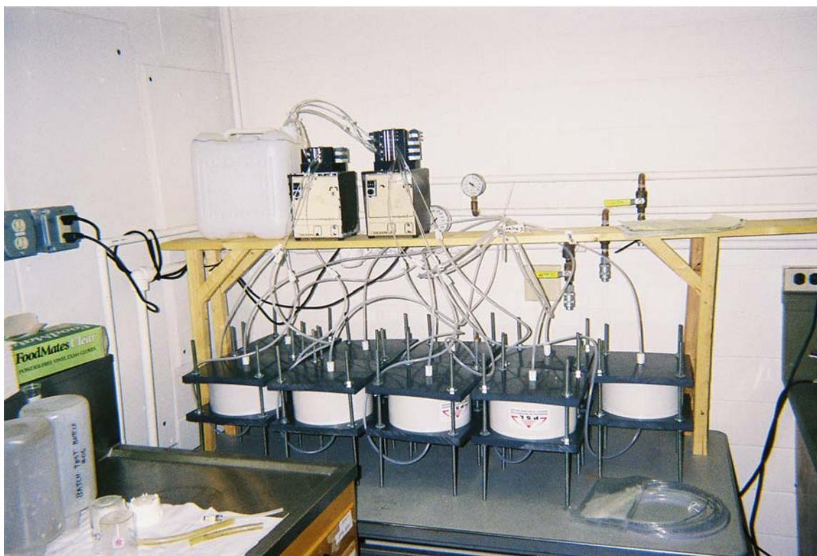
Fig. A-10. Column leach test on MnROAD materials.
