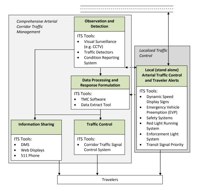
Figure 3: Illustration of ITS Tools that Support Arterial Traffic Management
